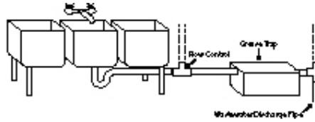
A grease trap is a box-shaped device that is connected to the drain line downstream of the three-compartment sink, prep sink, and mop sink. A vented flow control regulates the flow of wastewater through the grease trap and causes FOG and food solids to separate from wastewater. A series of baffles inside the device traps FOG and food solids while allowing wastewater to flow out of the trap.
