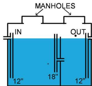
A grease interceptor is similar to a grease trap except it is much larger and is located in the ground outside of the kitchen. Gravity causes food solids and FOG to separate from wastewater. Baffles
