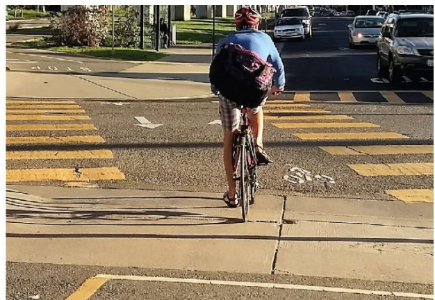
Figure 27: A high-visibility crosswalk with bike markings explicitly allows bicycles and alerts drivers to additional users.
