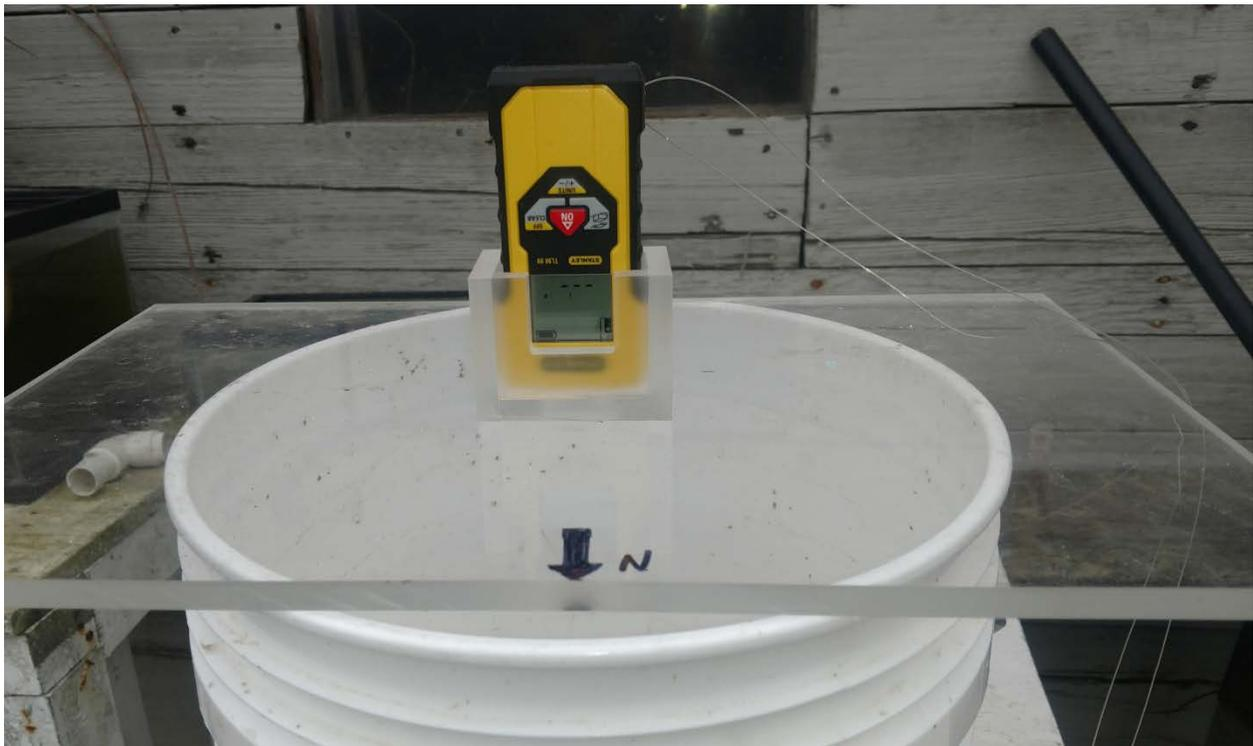
Figure 2- Plexiglass mount used for the TLM 99 laser measuring device. The mount has two marking, the visible “N” symbol and an “S” symbol on the opposite side. These two markings were made as a reference to take measurements from.
