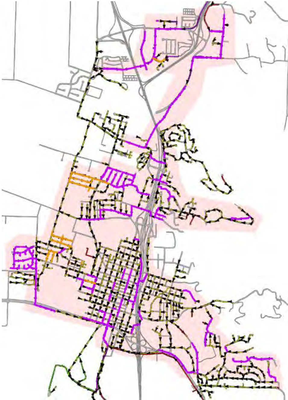
Figure 18 2018 I&I Reduction Project. Orange = Replaced Piping, Purple = Pipe Rehab via Lining.
