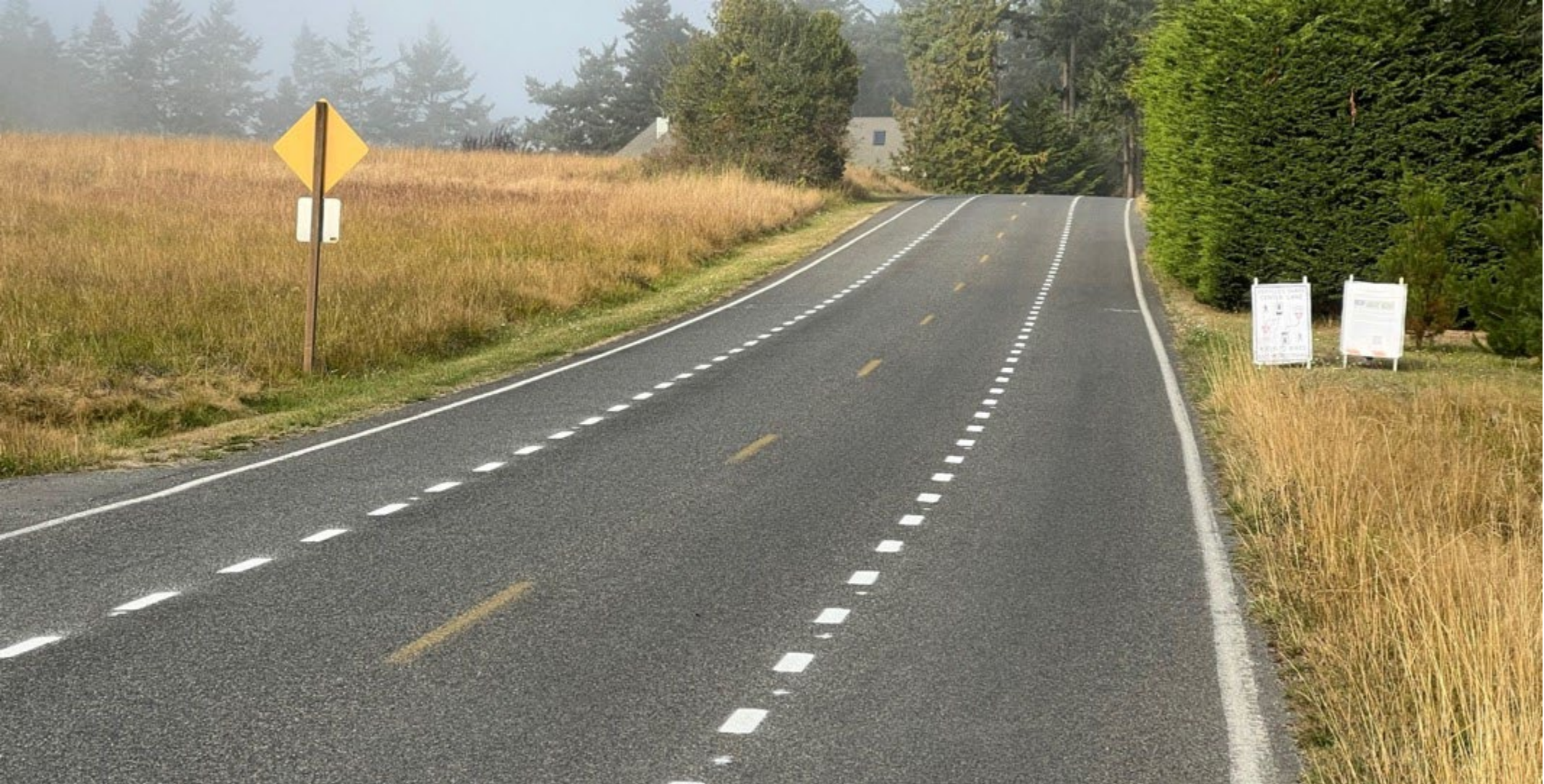
An example Edge Lane Road (Port Townsend, WA). Two-way Edge Lane Roads typically bring down speeds 2-7 mph, and increase safety for driving, walking and bicycling. Centerlines are removed or allowed to wear out.
