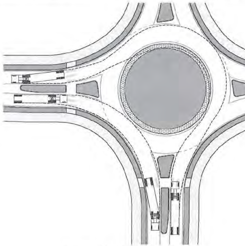
Figure 18. Design Vehicle Swept Path
