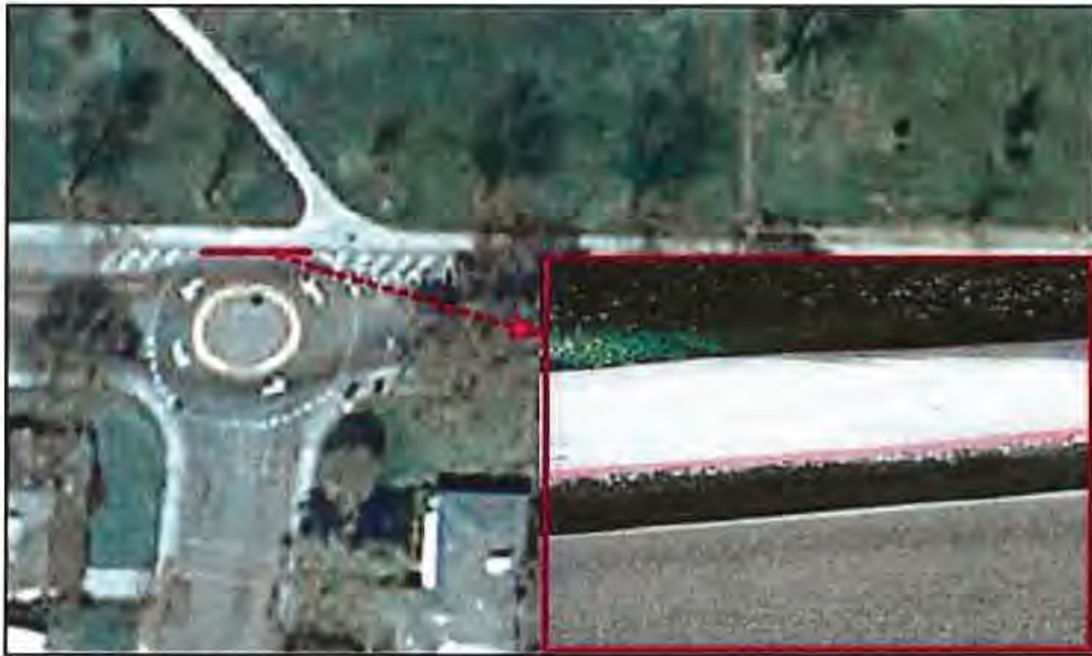
Figure 2. Inadequate Entry Deflection and Curb Damage at the Bowen Avenue/Phelps Avenue Roundabout in Modesto
