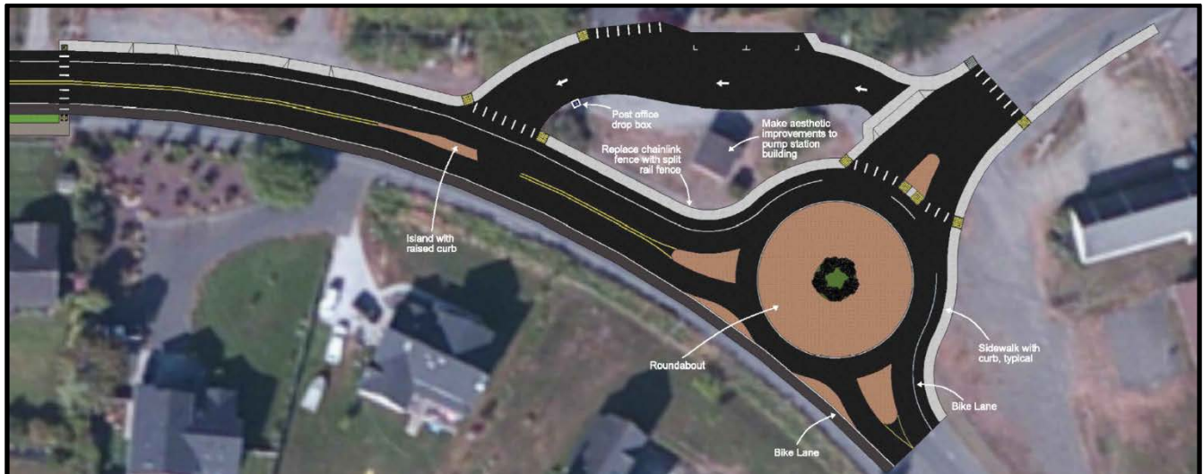
Figure 3.4 Proposed roundabout at the Jacoby Creek Road intersection. This option is presented in Alternatives Two and Four (SHN et al., 2017).
