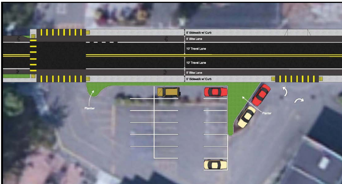
Figure 3.5 Proposed cross-section of the Jacoby Creek School Frontage with the proposed sidewalk option stated in Alternatives Three and Four (SHN et al., 2017).
