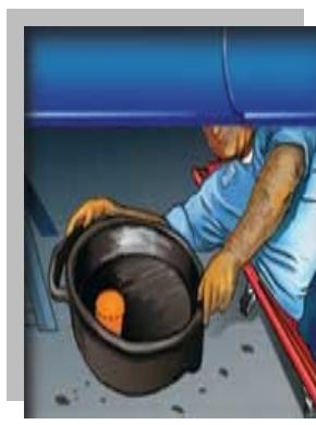
Place drip pans underneath to capture fluids. Use absorbent cleaning agents instead of water to clean work areas. Prevent fluid leaks from stored vehicles. Drain fluids such as unused gas, transmission hydraulic oil, brake
