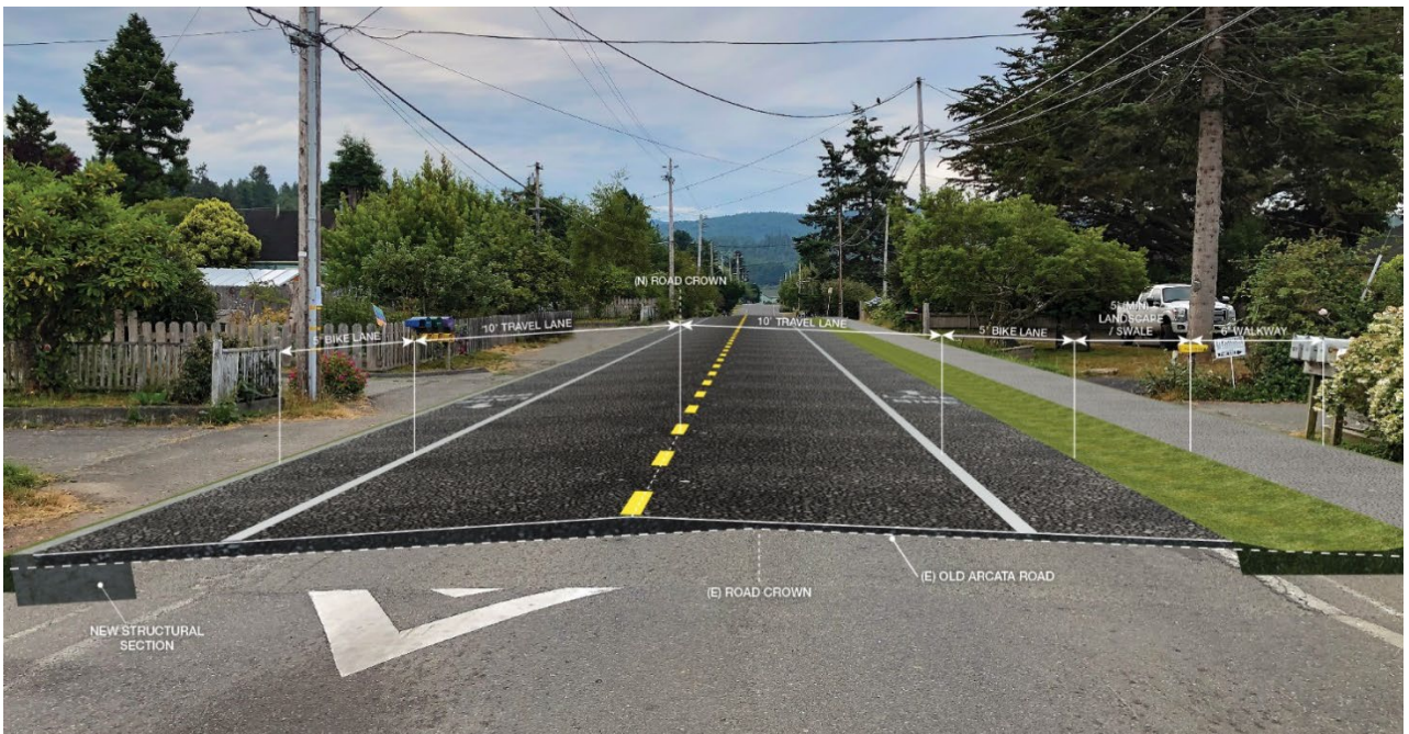
Exhibit 2: Comparative Rendering of Future Conditions of the Old Arcata Road Streetscape Showing Resurfaced Roadway, New Striping and Designated Bicycle Lanes, Stormwater Buffer, and Extended Pedestrian Walkway.
